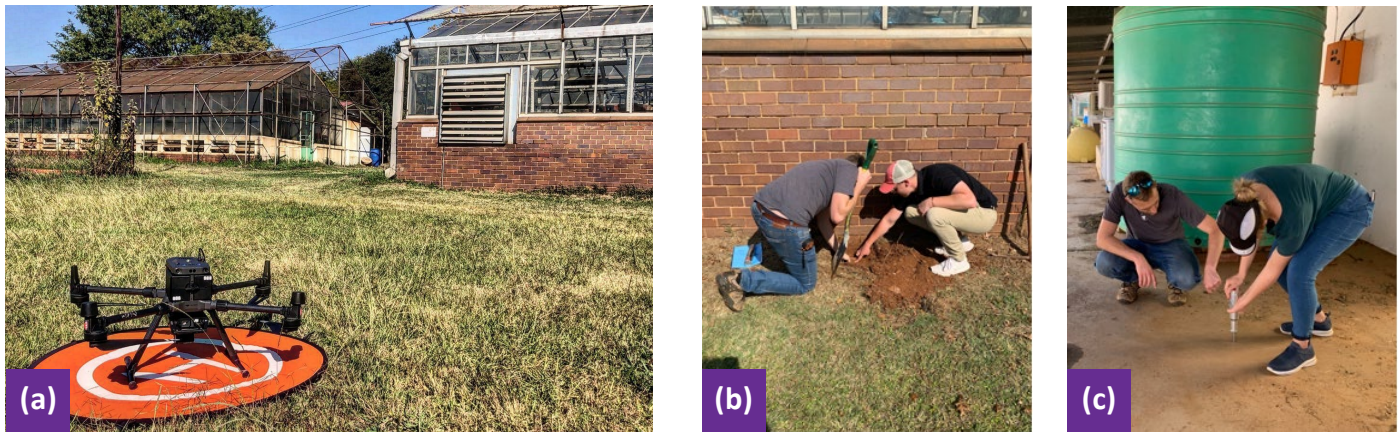
Figure 6: Capturing relevant information for the BIM model involved a range of different tools, ranging from drone operated LiDAR and photogrammetry (a), to non-destructive material testing (b), and simple pick axes and shovels to determine foundation sizes (c). (Davey, van der Merwe 2023).
