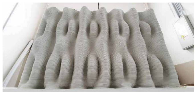
Figure 12: The 3D concrete printing modular walls, by, Luai Kurdi, 2019.
